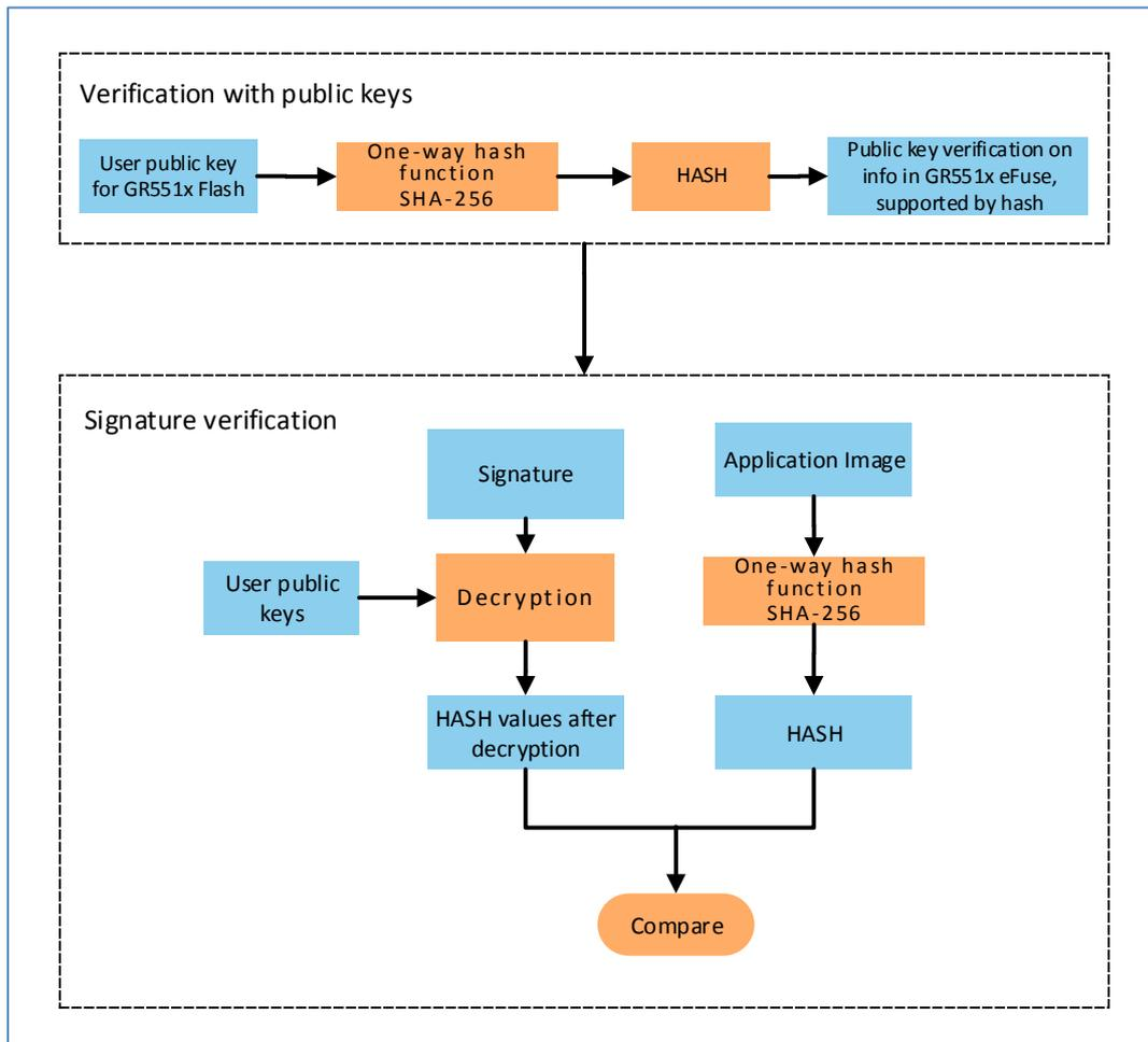
Figure 3-3 Verification process
