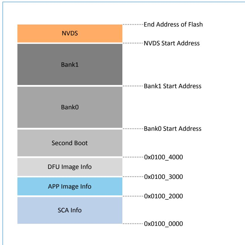
Figure 2-1 Flash layout of Second Boot example
