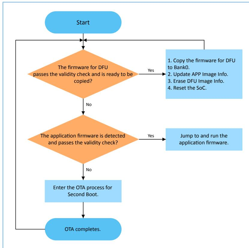
Figure 4-1 Process for running Second Boot example
