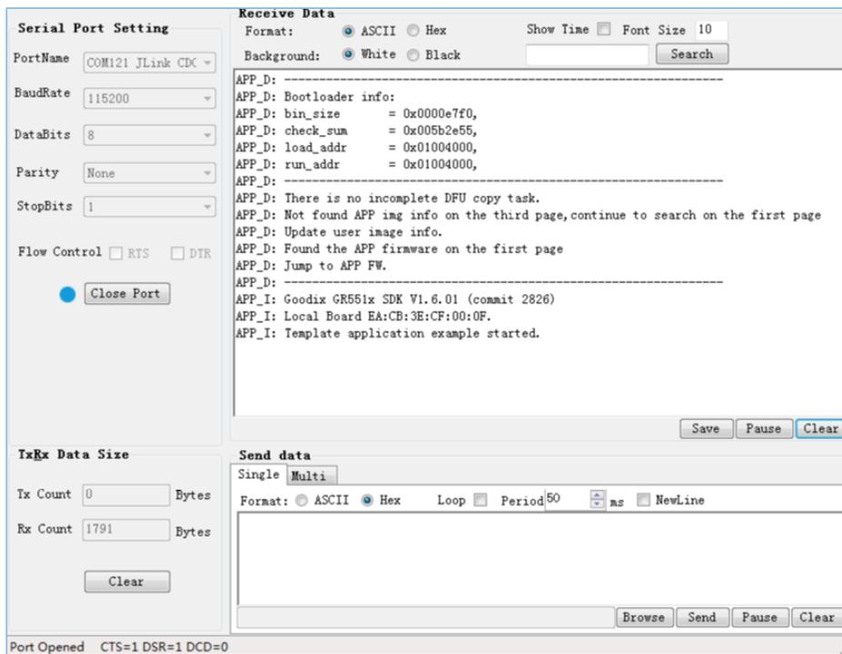
Figure 3-5 Application firmware running after successful update
