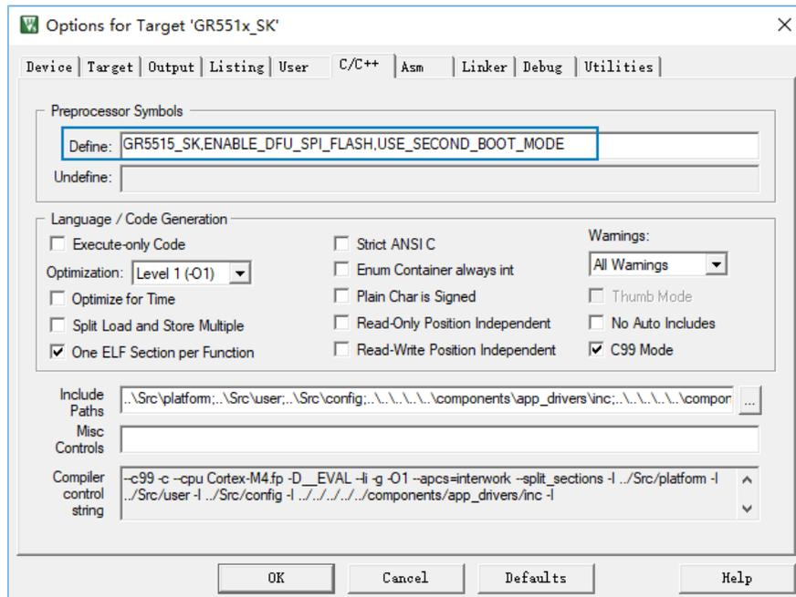
Figure 3-3 To enable the Second Boot mode
